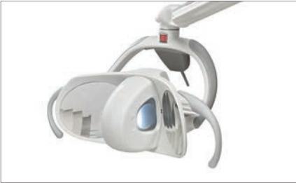
Maia LED light (optional) • Light intensity 45,000 lux, color temperature 5,000 K • Removable and autoclavable handles • 2-axis rotation
